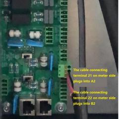
Figure 5 RS485 connections to the inverter
